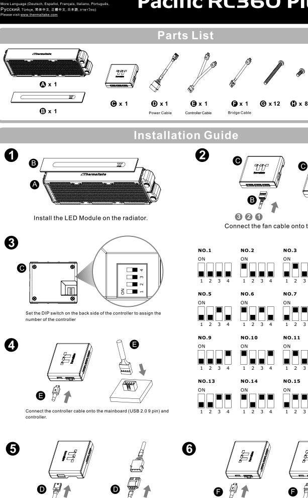
Connect the power cable to the 4pin Molex connecter and controller.
